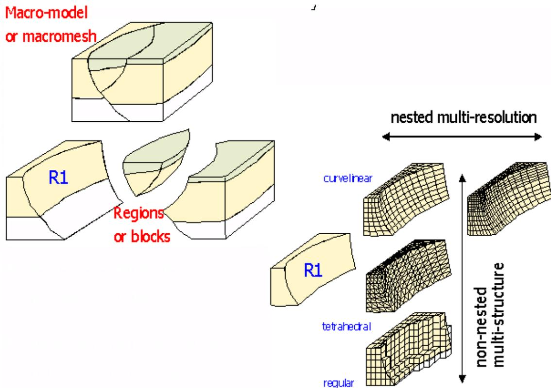
Figure 3 - MultiMesh toolkit concepts. See text for details.
