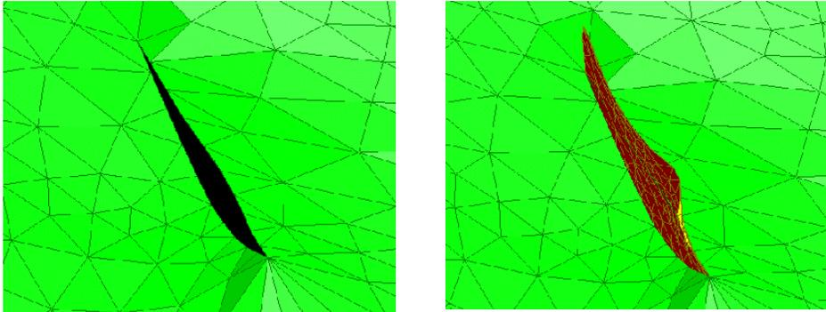
Figure 5 - A surface hole before and after the hole paving operation.
