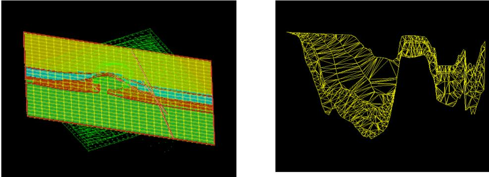
Figure 8- A) 2.5-D regularly gridded cross-section of a salt dome and B) triangulated cross-section of the Gulf of Mexico model displayed in Figure 4.
