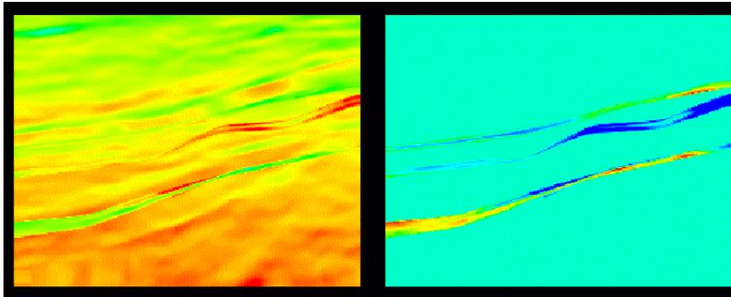
Figure 10 - Extraction of three reservoirs from 3-D seismic data.
