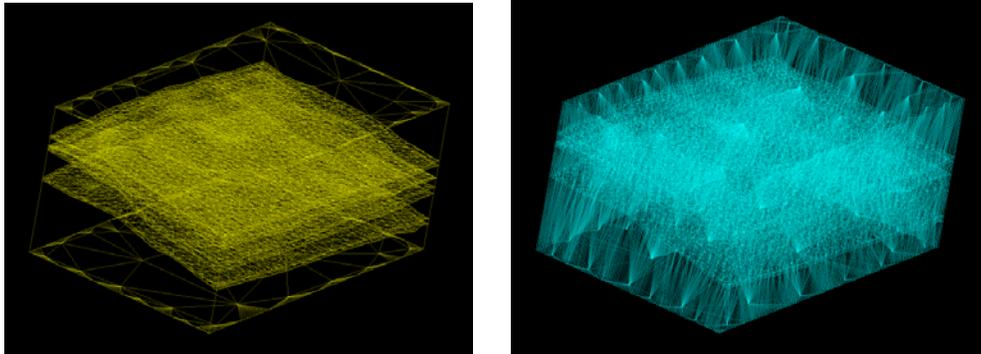
Figure 9 - Macromodel and tetrahedral mesh of a set of stacked reservoirs
