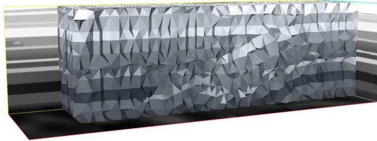
**Figure 5:** A cut of an atomic mesh obtained with the improved method.
